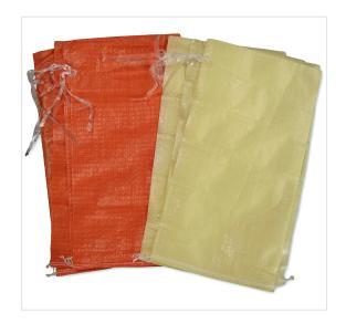
Our sandbags and gravel bags are manufactured with orange, light yellow, or white polystyrene strands. Strands have a typical thickness of 850 denier (weight for measuring the fineness of threads). Strand weave is typically 10x10 per square inch. Bags include zip ties or draw strings. Polystyrene strands are treated with UV inhibitors to accommodate up to 2,000 hours of UV protection.
